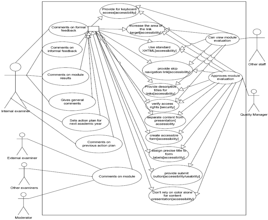
Fig. 2. The use case diagram of the online module review system after required accessibility considerations
