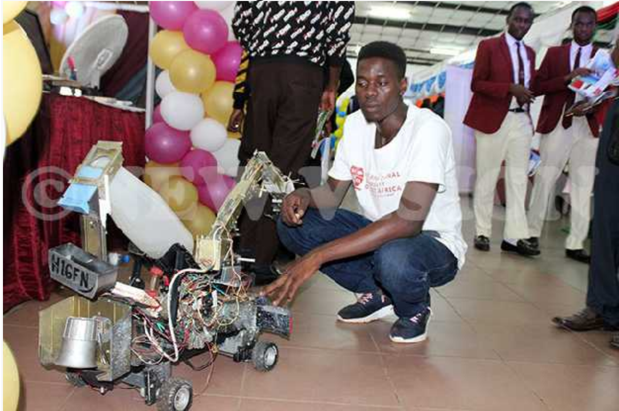
Horus Mwaka shows off his pesticide spraying robot. Photo by David Lukiiza
